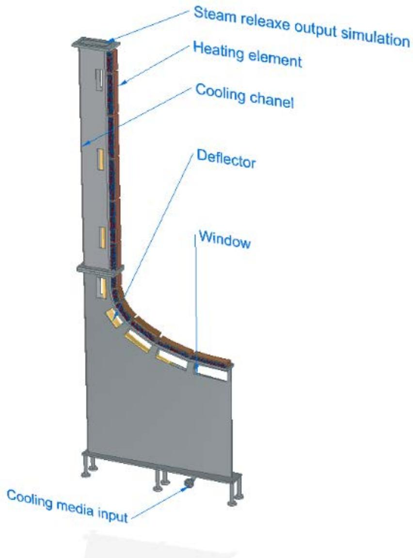
Fig. 6 Cooling channel basic design
