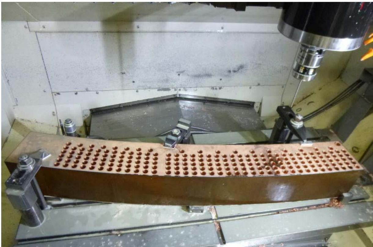
Fig.10 Heater segment with drilled holes.
