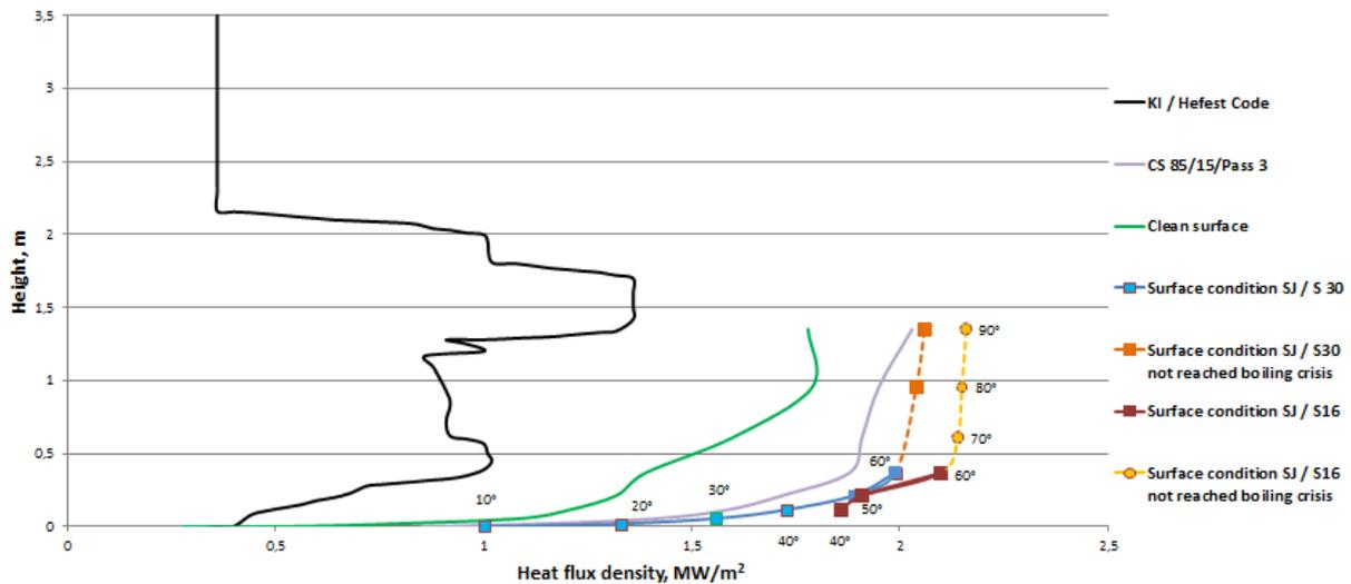
Fig.5. Summary of experimental results with different surface treatment.
