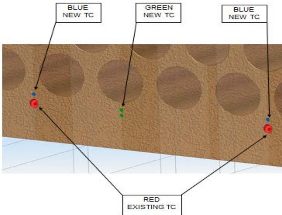
Fig.3. New thermocouple positions in the small scale sample.
