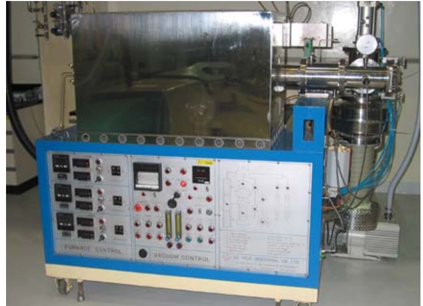
Vacuum Heat Treatment Furnace
