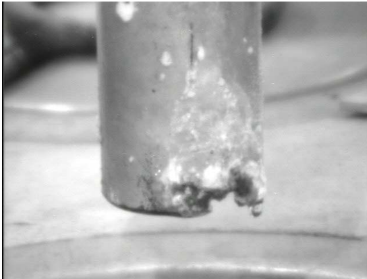
End fitting of fuel assembly stored on SS liner tube
