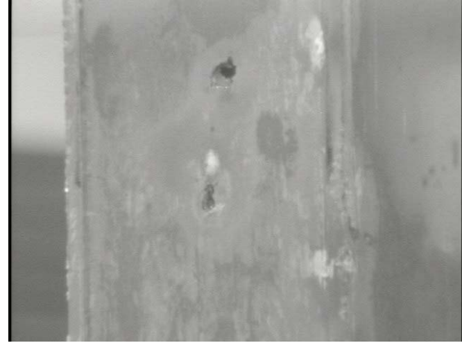
Corrosion pits with fuel meat exposure
