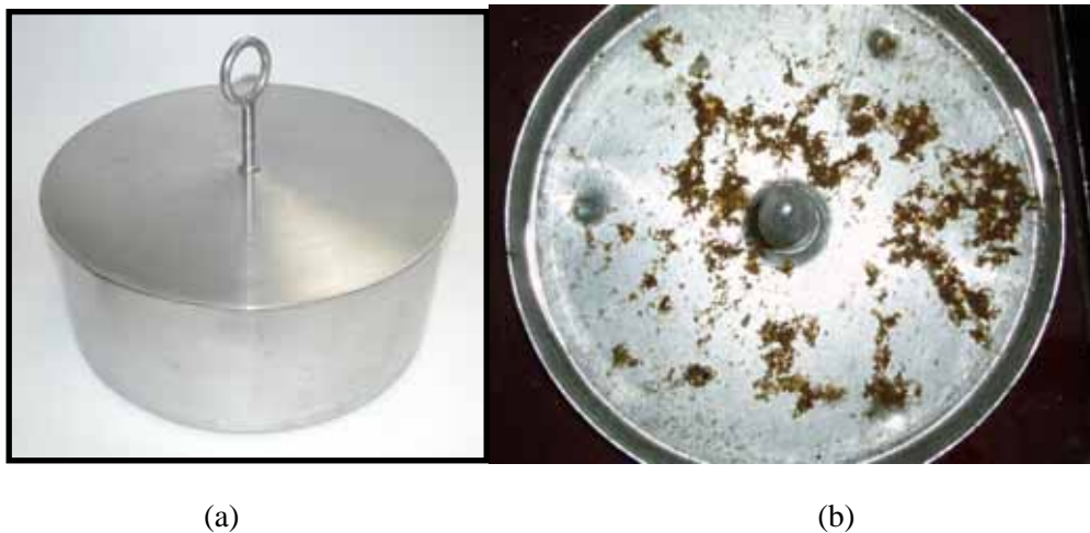
Fig. 1. (a) AISI 304 stainless steel collector used at CChen, Chile. (b) Settled solids in a collector
