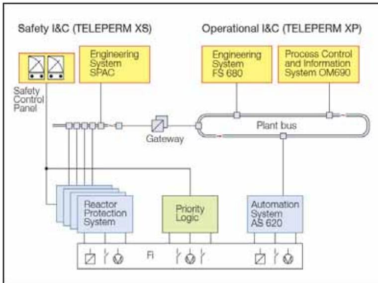
Figure 3. Tianwan I&C system structure
