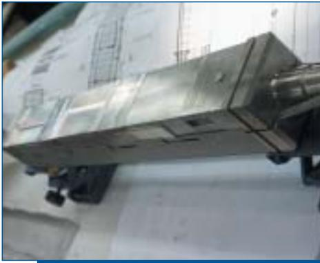
**Figure 2:** LYRA test rig for vessel metal irradiation in HFR.
