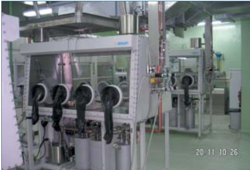
**Figure 3:** Globe box of the irradiation facility (IR-30) for spent fuel stability and pyrometallurgical separation of radionuclides studies.
