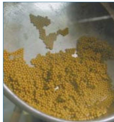
**Figure 1: first U Pu mixed oxide kernels manufactured in ITU.**
