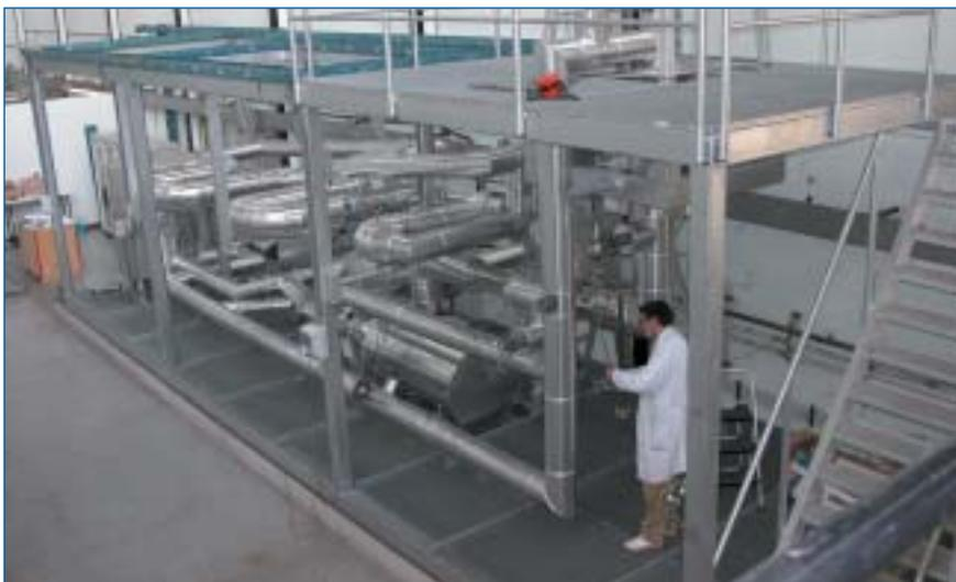
**Figure 1:** Pb-Bi loop for materials corrosion studies.
