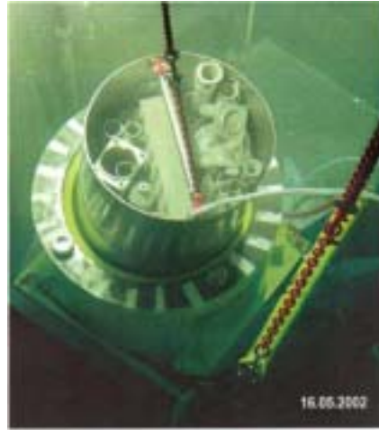
Fig 1. Conditioning of ILW – Under water loading of GNS-Mosaik Container
