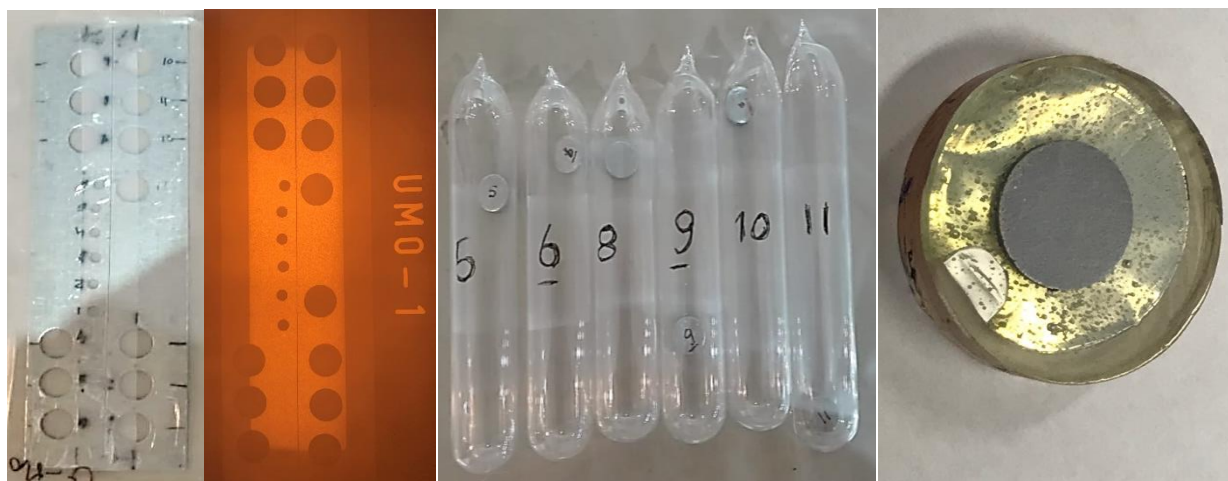
Figure 2. Photo and radiography of UMo/Al plate type target, punched for samples extraction. At centre, samples sealed in vacuum into quartz capsules and at right, sample mounted for SEM analysis
