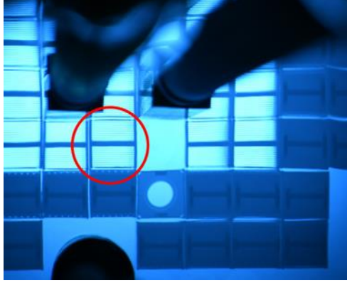
Figure 6. Irradiation of the FA intended for measurement (circled in red) next to a flux trap (lattice space filled with water, to the right of said FA) in the IRR-1 core.
