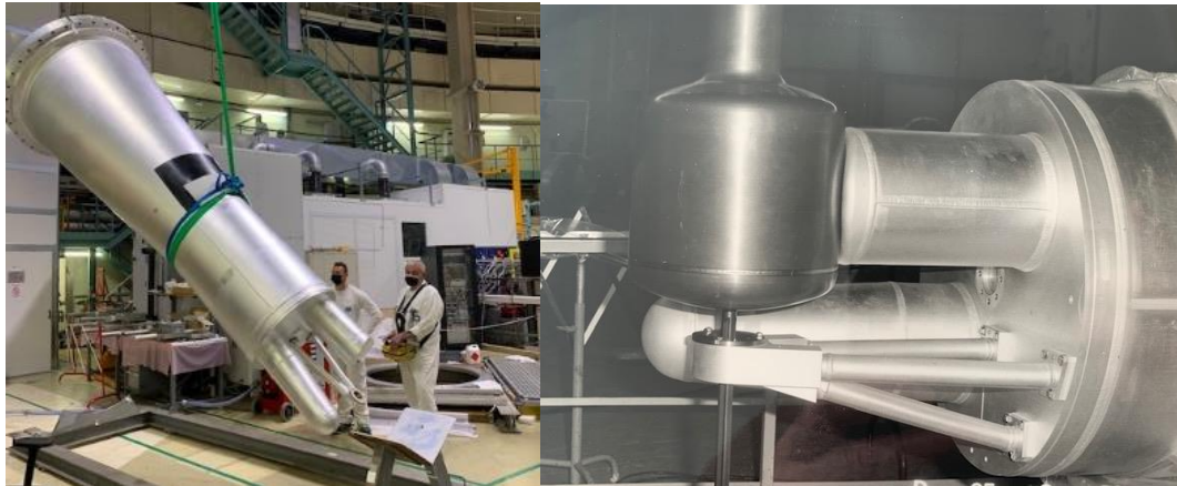
Fig 7. H1H2 beam tube with its cold source
