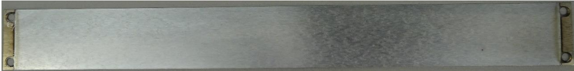
Fig. 6. Half-size foil after coating with the drilled und uncoated ends still to be cut.
