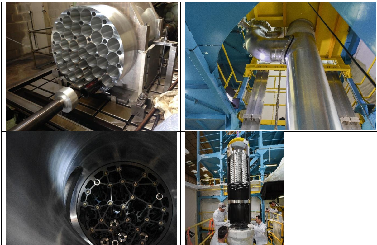
Figure 14: Manufacturing of reactor block components: core rack (VALLA), vessel and outlet of the primary circuit, top view of the upper grids and core rack, test lifting of the upper internals (CNIM)
