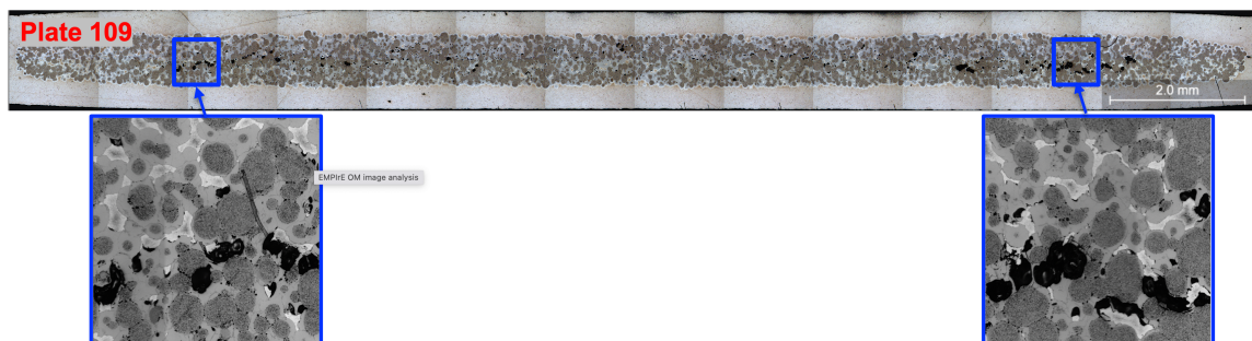
Figure 7. Cross-section montage of plate EMPI0109 showing the locations for the peak porosity measurement highlighted in blue.
