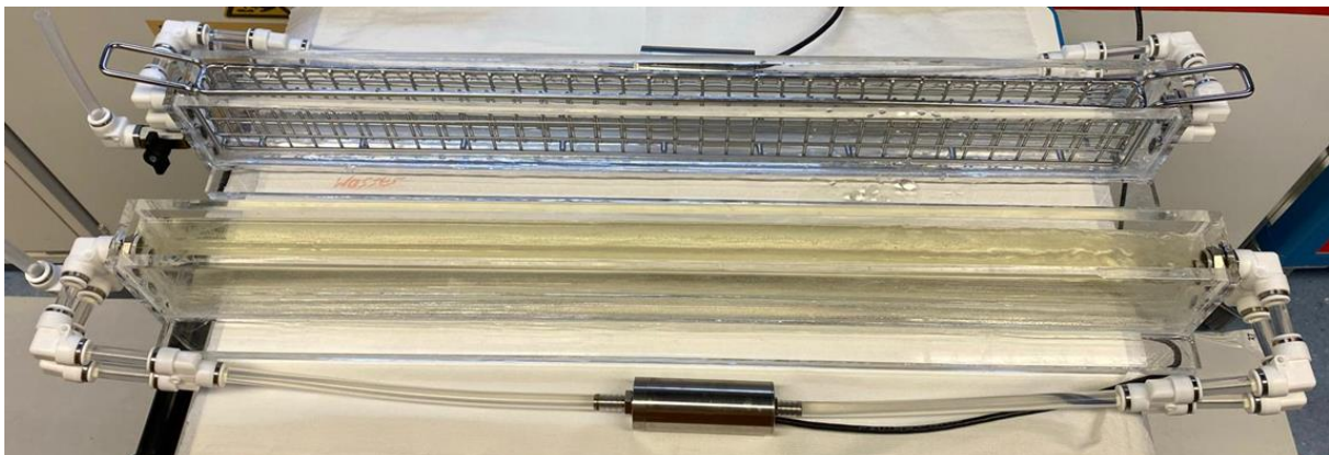
Fig. 4. Cleaning basins for full-size foils with circulation pumps. One filled with cleaning solution (front) and the other one with deionized water (back).
