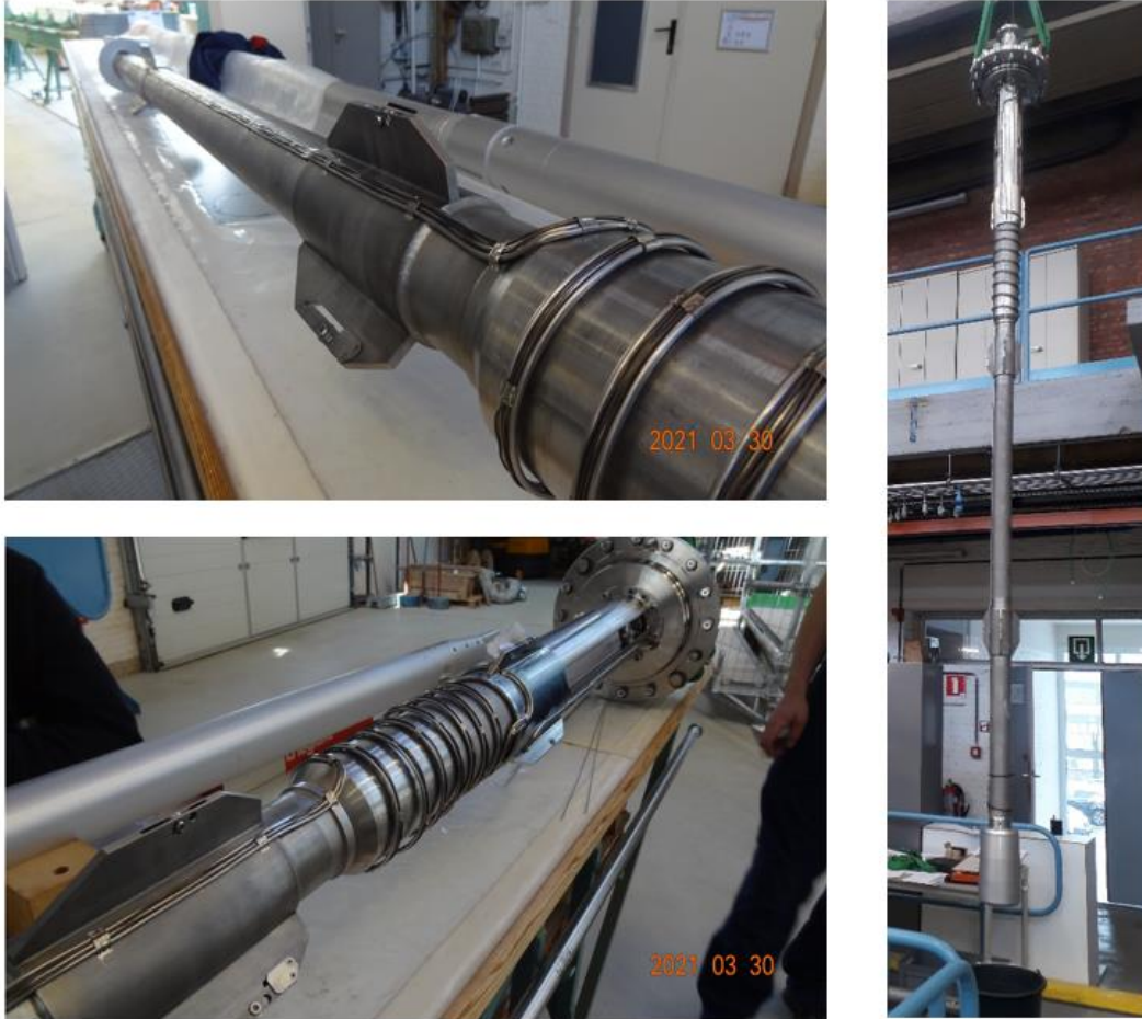
Figure 8 MUSTANG-R mock-up of restrictor suspension tube with plug (valve)
