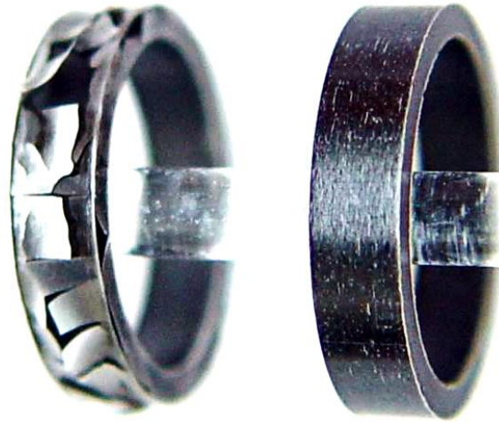
Figure 1: The two claddings after oxidation in high temperature steam. The E110 has spalling oxide layer (left), while the oxide on the E110G remains compact (right).
