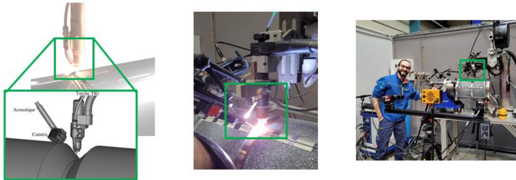
Figure 4 : Experimental set-up installation on RIS tube assembly at an industrial site.
